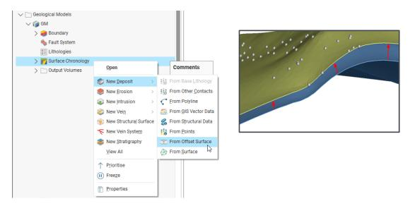
Maintains **consistent offset** while **honouring** contact points - for stratigraphy with common deformation
