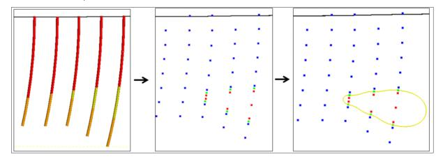
Can have **MULTIPLE** contact points per unit per borehole Intrusion volumes **enclose** the unit of interest
