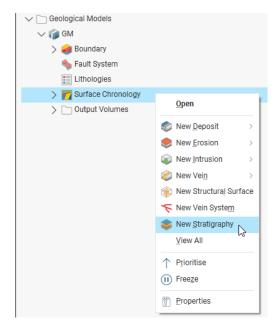
Generates multiple surfaces in a stratigraphic sequence in a single pass
