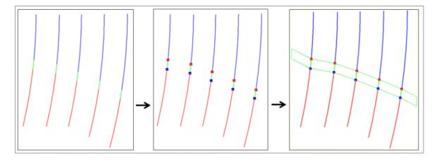
Creates a Hanging wall (HW) set AND Footwall (FW) set of contact points
