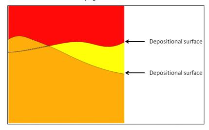
Deposit surface volumes cannot cut into an underlying older unit
